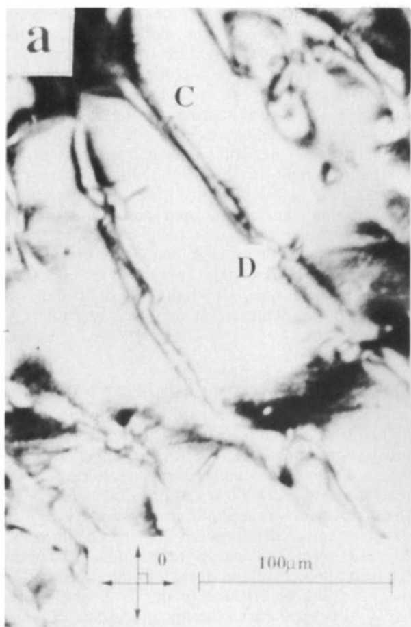
Figure 7 The contrast associated with the domain boundaries in a section of polymer 1, for two rotational settings of the crossed polars; the field alignment axis is from the top left to the bottom right of the figures
