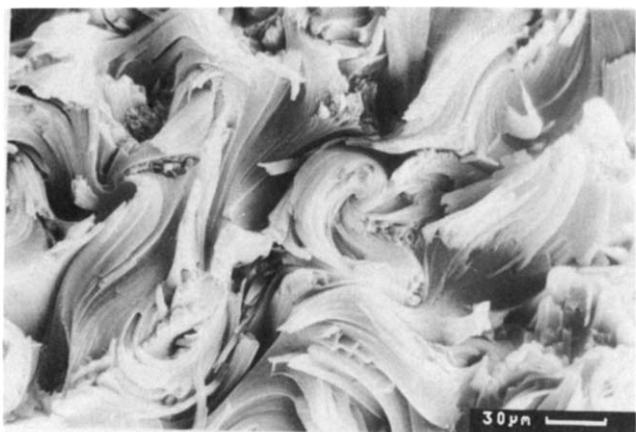
Figure 3 A scanning electron micrograph of the fracture surface of the sample shown in Figure 2
