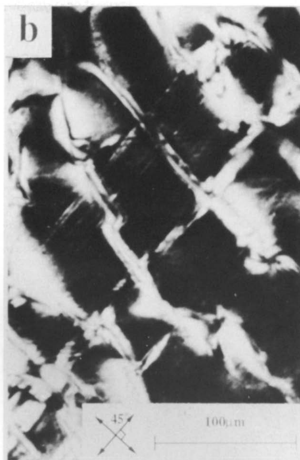
Figure 7 The contrast associated with the domain boundaries in a section of polymer 1, for two rotational settings of the crossed polars; the field alignment axis is from the top left to the bottom right of the figures
